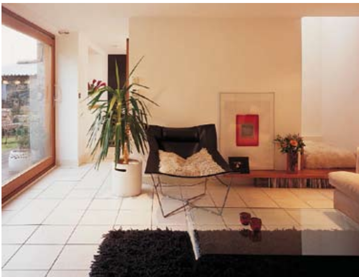
The sliding doors, which lead out onto a western red cedar deck, were created by a local joiner and feature Brazilian cedar frames.
